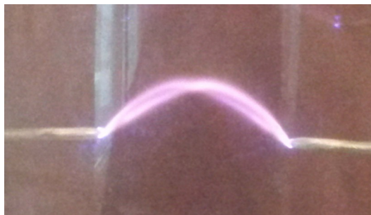
Fig. 1 Arc discharge in alternating current in the air with the pressure of 0.1 atm.
