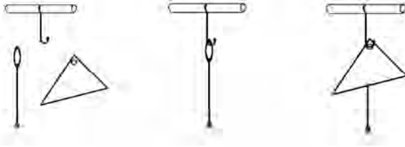
Fig. 3.21. Support with hook, plumb line and pierced pasteboard figure.
