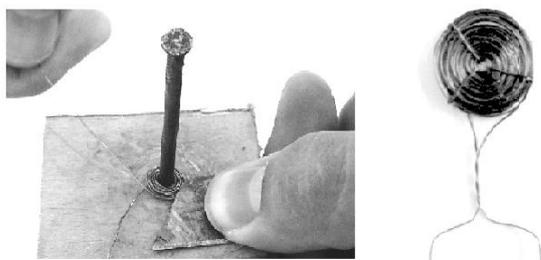
**Figure 4. Procedure to make the spiral and its final shape**
