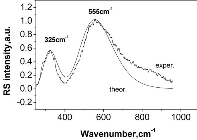
**Figure 7.** Comparison of the experimental and theoretical RS spectra for NaCl:KBF<sub>4</sub> (5.7% Na). The theoretical spectra were obtained using  $\sigma = 0.5$  nm,  $d_0 = 6.5$  nm, resulting in  $\nu_0 = 582$  cm<sup>-1</sup> (for the  $\nu_{\max} = 550$  cm<sup>-1</sup> peak). For the  $\nu_{\max} = 325$  cm<sup>-1</sup> peak we obtain  $d_0 = 8.5$  nm, and  $\nu_0 = 335$  cm<sup>-1</sup>; the experimental curve was normalized and this was followed by a baseline subtraction.
