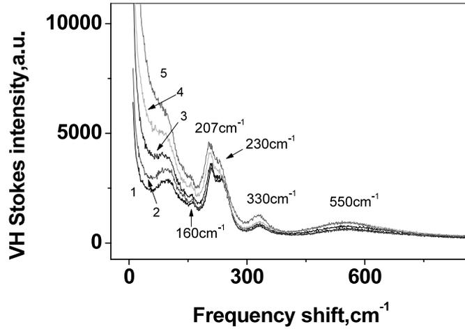
**Figure 1.** The Raman VH spectra of heavily electron irradiated crystal NaCl:K (sample 2,  $T_{irr} = 110^\circ\text{C}$ , 150 grad with 3.6 mol% Na); the measuring temperatures are: 1: 30; 2: 50; 3: 100; 4: 150; 5: 200 K.
